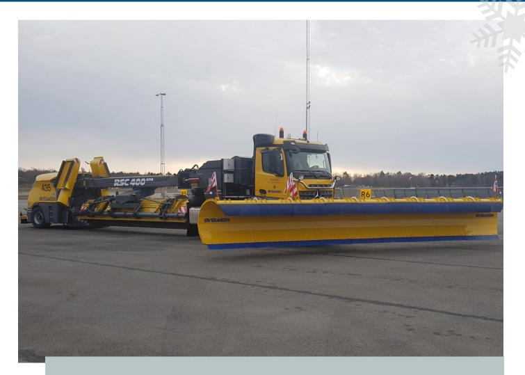
The ØVERAASEN RSC 400 Performance Line is designed as a 6x4 vehicle built on a standard truck chassis. The machine offer the highest degree of maneuverability and clearing capacity. The biggest advantages of the Øveraasen RSC 400 compact runway sweeper are the compact design, the flexibility and the high working speed. This makes Øveraasen RSC 400 unique for the market for unlimited use on runways, taxiways and aprons.
